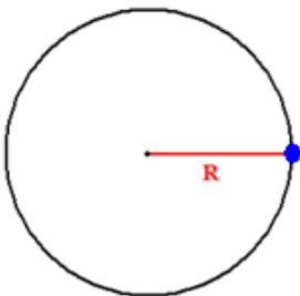
If we rotate the disk  $x$  number of radians, what distance will the sticker travel? Well, we know by the definition of a radian, for every radian rotated, the sticker is going to travel an arc length equal to one radius of distance.
