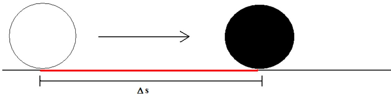
Clearly, the length of the red line is one circumference of distance, or  $2\pi \cdot R$ . The cylinder itself make one complete rotation, so its angular displacement was  $2\pi$  radians.
