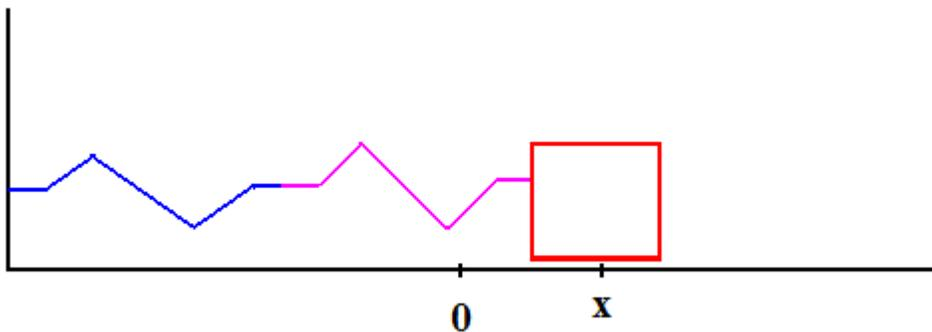
We know that  $x$  in this diagram is the sum of the stretching of the two springs, which we can call  $x_1 + x_2$ . We can then rearrange Hooke's law into  $x = \frac{-F}{k}$ .
