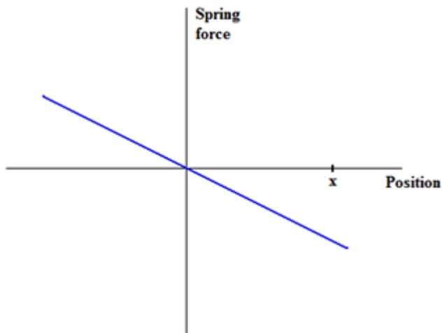
Again, you can see that when the box has a negative position, the spring applies a positive force (in the second quadrant of the graph) and when the box has a positive position, the spring applies a negative force (in the fourth quadrant of the graph).
