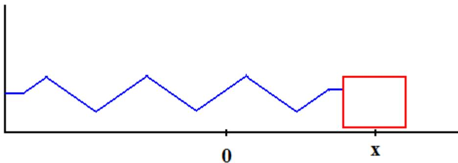
For many springs, the force the spring pulls back to the left with increase as  $x$  increases. The more the spring is stretched, the harder it pulls back leftward with a negative force.
