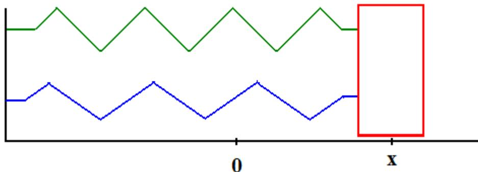
The top spring will apply a force of  $-k_1 \cdot x$  on the block, the bottom spring will apply a force of  $-k_2 \cdot x$  on the block, making the net force on the block  $(-k_1 \cdot x) + (-k_2 \cdot x)$ .
