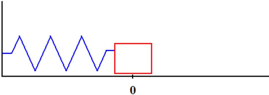
If the spring is neither compressed nor stretched, we will define the position of the block to be zero. We can then pull the block to the right to a position  $x$  and use a force-meter to determine the force that the spring applies when stretched this amount.
