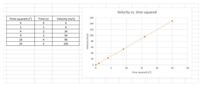
Now this is a linear function we can work with. The slope is 6 and the y-intercept is zero, so:  $v = 6t^2$  and that's it. That's the function of the first graph we were looking for.
