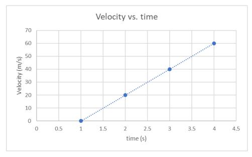
For instance, the graph above has a slope of  $20\text{m/s}^2$  and an *x-intercept* of 1s, but we still need the *y-intercept* to use the form y = mx + b. Well, just solve for it. When y = 0, x = 1, so:
