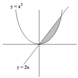
We can then calculate the left and right boundaries of this shaded area with  $x^2 = 2x$  so that  $x_1 = 0$  and  $x_2 = 2$ .
