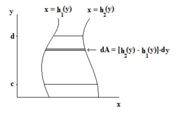
$$V = \int_{c}^{d} \int_{h_{1}(y)}^{h_{2}(y)} f(x, y) \cdot dx \cdot dy$$
